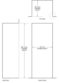
NOTE: 3<sup>1</sup>/2\* (89) finished returns will be visible and should be finished to match cabinetry.
