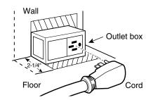
Recommended acceptable electrical outlet area. Orient the electrical receptacle so the length is parallel to the floor.
