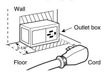
Recommended acceptable electrical outlet area. Orient the electrical receptacle so the length is parallel to the floor.
