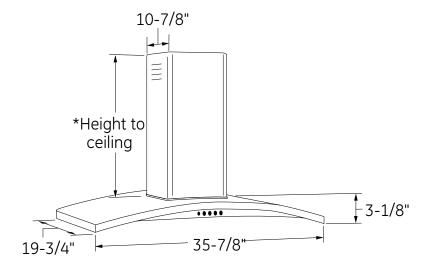
\* The supplied duct cover fits 7'11" to 9'7" ceiling heights (10' in recirculation mode).
