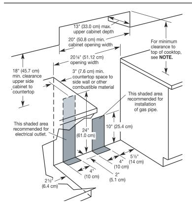
**NOTE:** 24" (61 cm) minimum when bottom of wood or metal cabinet is covered by not less than ½" (0.64 cm) flame retardant millboard covered with not less than No. 28 MSG sheet steel, 0.015" (0.4 mm) stainless steel, 0.024" (0.6 mm) aluminum or 0.020" (0.5 mm) copper. 30" (76.2 cm) minimum clearance between the top of the cooking platform and the bottom of an uncovered wood or metal cabinet.
