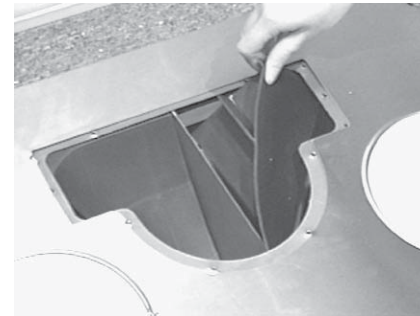
3. Remove 2 air diverter blocks through top opening as shown.
