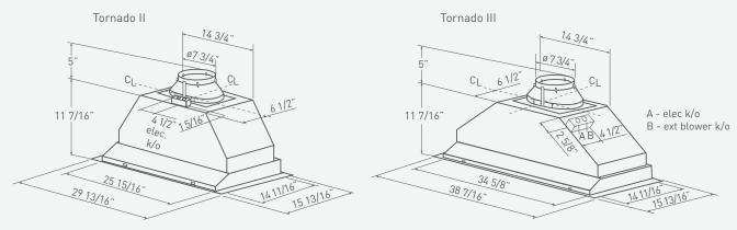
Cabinet Bottom Cut-Out Size (W x D): AK8200AS: 26 1/16" x 14 3/4"; AK8300ASX: 34 11/16" x 14 3/4"
