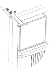
14. Place the door latch assembly on opposite side of unit. Be sure to tighten all three screws securely.
