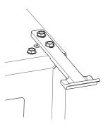
15. Place door on lower hinge pin. Invert and install upper hinge on door. Fasten upper hinge to unit (three screws). Partially tighten screws.
