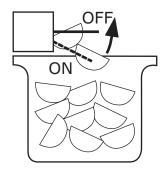
**To turn off ice production:** Raise the bin arm into an upright and locked position. The unit will preserve temperature for ice storage.
