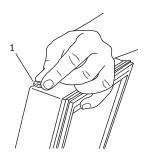
8. Using a Phillips screwdriver, remove the two screws holding the custom stainless handle from the original location and remove the handle. Remove the two screws on the opposite side of the door. Do not place handle on door until you have completed steps 9 and 10.
