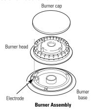
2. Place the burner cap on top of the burner head. Make sure that the burner cap is properly seated on the burner head.
