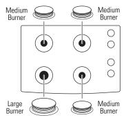
On model ZGU384, there is one large burner head and burner cap and three sets of medium burner heads and burner caps.
