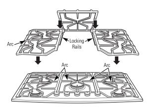
**Model ZGU385:** Replace the two side grates with their locking rails toward the center grate so that a continuous "arc" is formed with the center ribs of all three grates. Make sure the center grate is locked into position over the rails on the side grates and that all grates are stable and level.
