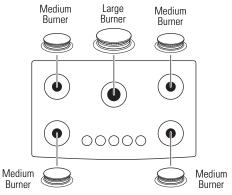
On model ZGU385, there is one large burner head and burner cap and four sets of medium burner heads and burner caps.
