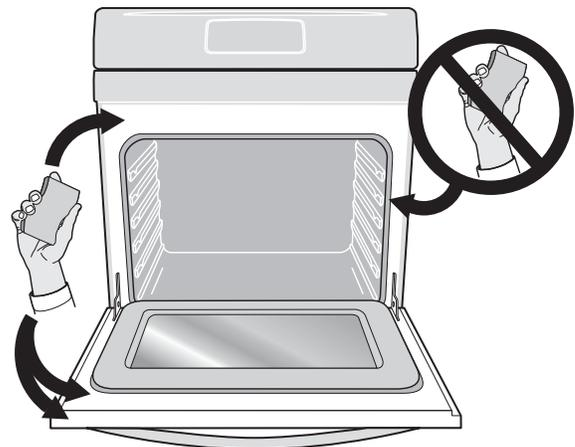
Figure 11: Clean around the oven door gasket
