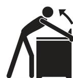
To check if the anti-tip bracket is installed properly, use both arms and grasp the rear edge of range back. Carefully attempt to tilt range forward. When properly installed, the range should not tilt forward.
