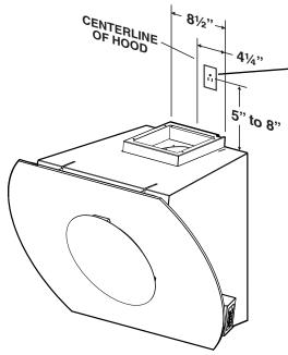
120 VOLT 60 HZ GROUNDED WALL OUTLET OFFSET FROM DUCT CENTER LINE (STAY WITHIN 41/4" DIMENSION)
