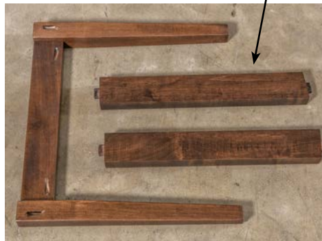
leg assembly glued & pocket-screwed
