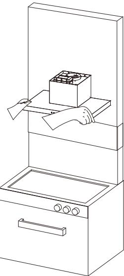
Then fix the body on (A,B) holes to the wall using the screws.
