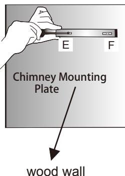
Screw the chimney mounting parts into Ø 8mm sized wall plugs on E,F points which is provided with your product.
