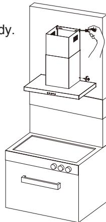
Screw internal chimney on chimney fixing sheet, fixed over upper corner of external chimney.
