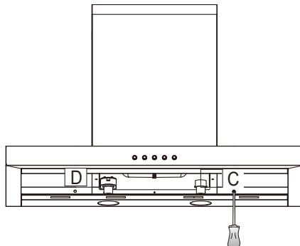
**NOTE:** If the hood seems to be tilting, slightly loosen the screws that are used on the hanging parts at the top and straighten until the hood is vertical.
