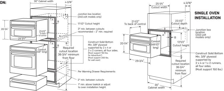
A / B = Allow the following clearances around the cutout on the front surface of the cabinet: 1.7/8" from the top, 2.3/8" from the side edges and 1.1/8" from the bottom. **NOTE:** these refer to minimum clearances required for installation and do not reflect actual product dimensions.
