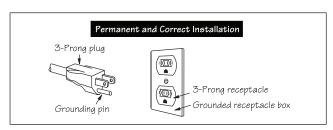
AWARNING Improper use of the grounding plug can result in a risk of electric shock. Do not use an extension cord. If the power supply cord is too short, have a qualified electrician or serviceperson install an outlet near the appliance.
