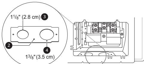
For power cord ⑤ installations, hook the strain relief over the power cord hole (1 3/8") located below the rear of the oven.
