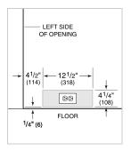
**NOTE:** The electrical outlet must be positioned with the grounding prong to the right of the thinner blades
