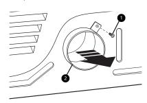
2 Press the tabs on the knockout ③ and carefully remove the knockout for the desired vent opening. (Right-side venting is not available on gas models.) Press the adapter duct ④ onto the blower housing and secure to the base of the dryer as shown.
