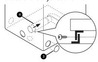
Preassemble a 4" (10.2 cm) elbow to the next 4" (10.2 cm) duct section, and secure all joints with duct tape. Be sure that the male end of the elbow faces AWAY from the dryer. Insert the elbow/duct assembly through the side opening and press it onto the adapter duct. Secure it in place with duct tape. Be sure that the male end of the duct protrudes 1.5" (3.8 cm) to connect the remaining ductwork. Attach the cover plate to the back of the dryer with the included screw.
