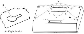
2. Use  $\frac{1}{8}$ " (3 mm) drill bit and drill 4 pilot holes as shown.
