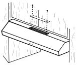
**NOTE:** For installations which are venting out the roof or wall, **the recirculating vent cover must remain in place**.
