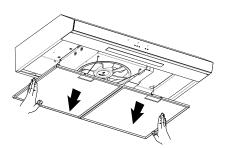
Remove the grease filters
