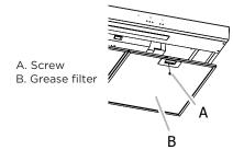
2. To remove, pinch the filter latch and pull down the front edge.
