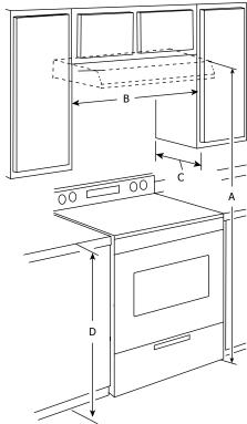
A. 66" (167 cm) suggested min. - top of range hood to floor. B. 30" (76.2 cm) min. cabinet opening width for 30" (76.2 cm) models and 36" (91.4 cm) min. cabinet width for 36" (91.4 cm) models.
