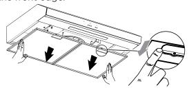
3. Remove carbon filter rods and remove carbon filter (located on the back of the grease filter).
