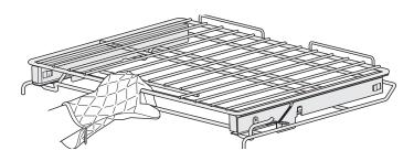
While holding both sections, pull the glide rack out of the oven until the stop position is reached.
