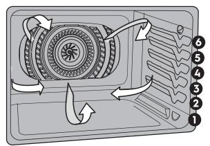
Figure 6: Convection roasting on lower oven racks
