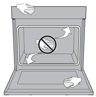
Figure 7: Clean around the oven door gasket
