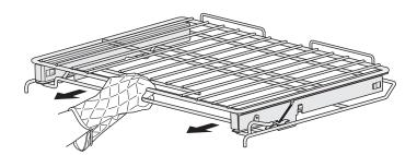
Using both hands, lift up the front of the rack slightly and continue to pull the rack away from the oven. Be sure to grasp both upper and lower rack portions together when removing or handling the glide rack.
