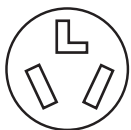
3-wire receptacle (10-30R)
