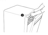
Align the dishwasher with the opening. Make sure the water supply line and electrical cable are in the correct positions to slide into their channels properly.
