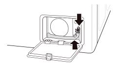
7 Insert the drain pump filter and twist it clockwise.
