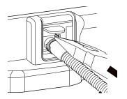
Screw in the band to secure the drain hose of the dryer onto the stacking bracket.
