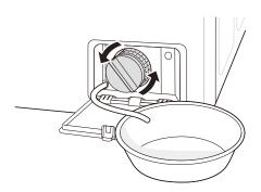
Clean the pump filter and opening.
