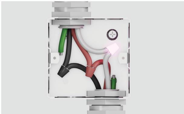
1. Separate the green and white oven cable wires. Connect the white oven cable wire to the neutral (white) wire in junction box.
