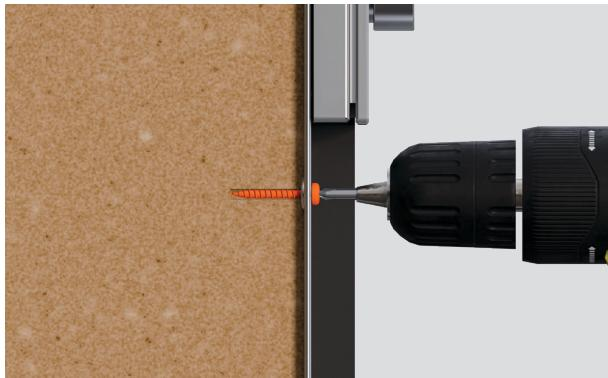
2. Secure oven to cavity using the 2 x screws provided.
