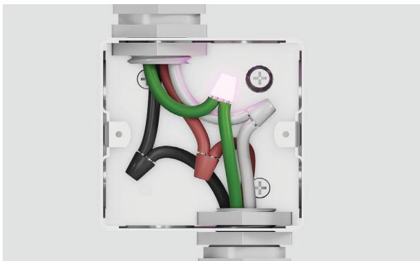
2. Connect the green grounding oven cable wire to the (green) grounding wire in the junction box. Do not connect the green grounding wire to the neutral (white) wire in junction box.
