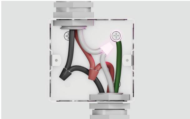
1. Separate the factory-taped green and white oven cable wires. If junction box is grounded, connect the green wire to the metal junction box with a screw before connecting the white oven cable wire to the neutral (white) wire in junction box.
