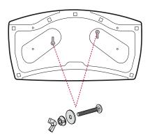
2-Screws for Stand Fixing, 2-Washers for Stand Fixing, 2-Nuts for Stand Fixing (Provided as parts of the product.)
