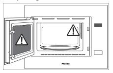
There is a cover protecting the microwave outlet on the right-hand side of the oven compartment and a layer of film protecting the inside of the door, both of which are susceptible to damage.
