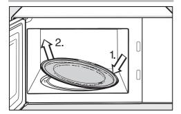
Do not turn the turntable manually, as this could damage the drive motor.
