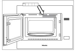
■ Attach the enclosed quick guide to the frame behind the door (as illustrated), making sure it does not block any of the vents.
