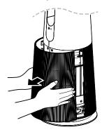
3 Remove the filter and dispose of the packaging.
