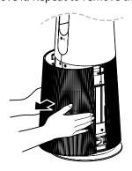
Using a vacuum cleaner or soft brush, remove any dust from the ultra-fine filter surrounding the filter.
