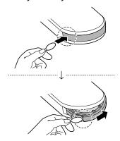
3 Insert the battery in the tray with the + polarity facing up.
