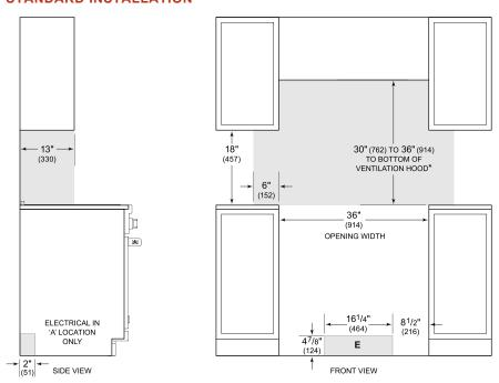
†Without ventilation hood, 36" (914) minimum clearance countertop to combustible materials. NOTE: Shaded area above countertop indicates minimum clearance to combustible surfaces
