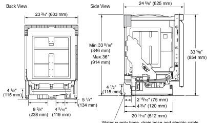
Water supply hose, drain hose and electric cable should be passed through this area.
