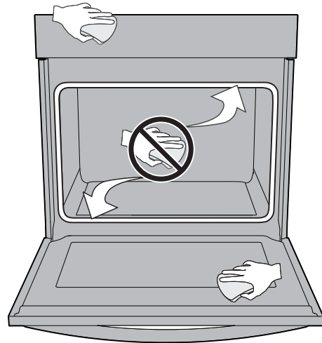
Figure 11: Clean around the oven door gasket
