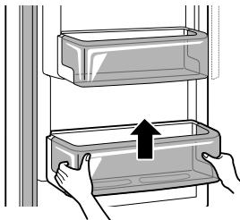
**2** To assemble the bin, slide it in above the desired support and push down until it snaps into place.
