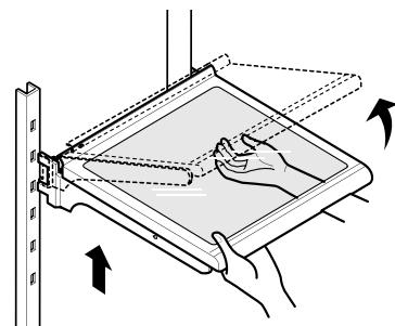
**5** To assemble, tilt the front of the shelf up and guide the shelf hooks into the slots at a desired height.
