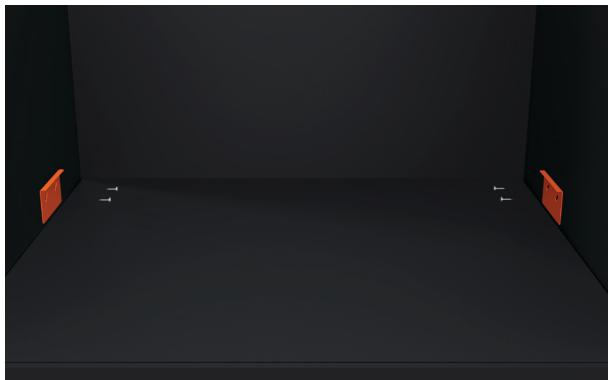
1. Position the anti-tip brackets on both sides of the cabinetry. Brackets should be located flush to the base of the cabinet and 15 3/16" (385mm) from the front of the cabinet for Minimal and Contemporary models and 14 15/16" (380mm) for Professional models.
