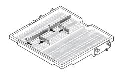
Pull tines back up to fit smaller dishes.
