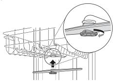
After assembly, make sure that the spray arms rotate freely.
