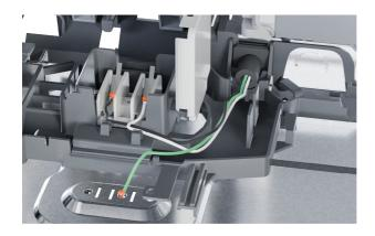
5. Unscrew the Live (black), Neutral (white) and Earth (green) wires from the terminal block and the chassis.
