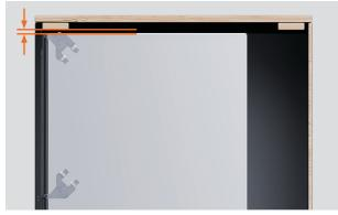
**3.** Adjust the dishwasher height to 1/8 to 3/16" below the cavity height.
