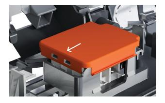
**4.** Slide the terminal block cover sideways to unlock and hinge open to access the terminal block.
