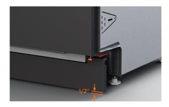
**4.** Snap off the top tabs. Slide the pre-finished toe kick along the T rails into position. Ensure there is a 1/2" gap between the toe kick and the floor.
