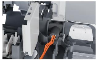
**6.** Safely cut the cord from the inside **and outside** of the strain relief molding to remove the cord.
