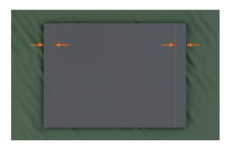
**3.** Use the final measurements to mark vertical lines on the back of the custom panel.
