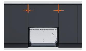
**2.** Subtract the required gap between the cabinet panels from each measurement.
