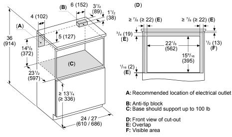
If under a counter, minimum clearance to counter top should be  $^{7}/_{16}\text{"}$  (11 mm)
