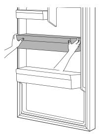
**2** To assemble the bin, slide it in above the desired support and push down until it snaps into place.
