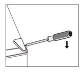
2.Undo the screws.Then remove the hinge bracket.
