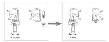
7. Refit the bracket fitting the bottom hinge pin. Replace both adjustable feet.
