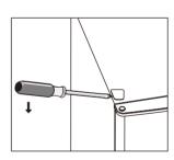
4. Move the core cover from left side to right side. And then lift the upper door and place it on a padded surface to prevent it from scratching.
