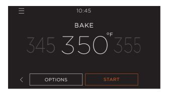
**4.** Adjust the temperature if needed, then press **START**.
