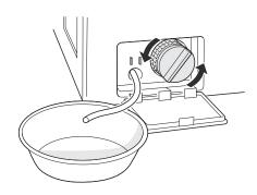
Clean the pump filter and opening.
