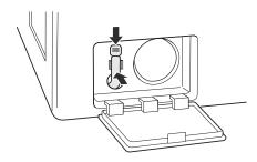
Insert the drain pump filter and twist it clockwise.
