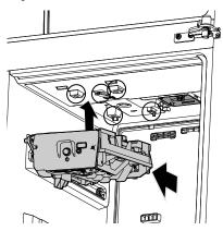
5. Plug the ice maker's electrical connector into the mating connector in the ceiling of the freezer. Wrap the wire around and through the hooks as shown in the image below. The wire must be pulled tightly to hold in the hooks.
