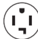
4-wire receptacle (14-30R)
