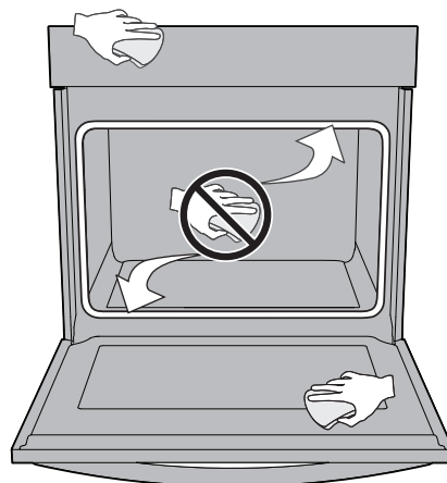
Figure 16: Clean around the oven door gasket
