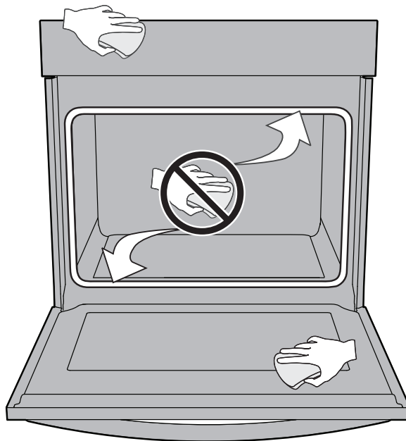
Figure 14: Clean around the oven door gasket
