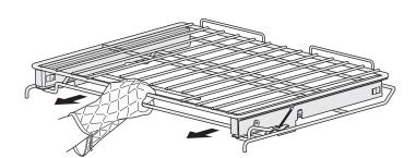
Using both hands, lift up the front of the rack slightly and continue to pull the rack away from the oven. Be sure to grasp both upper and lower rack portions together when removing or handling the glide rack.
