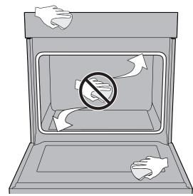
Figure 6: Clean around the oven door gasket
