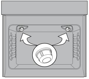
Figure 10: Wall oven Halogen light
