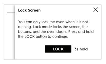
Touch and hold **LOCK** for 3 seconds. You will be shown a code to use for unlocking the doors and controls. This ensures that the oven will remain locked and safe.
