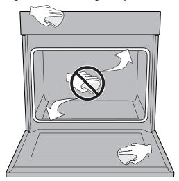
Figure 8: Clean around the oven door gasket
