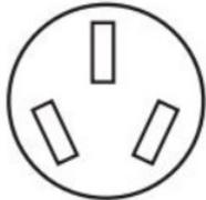
3-wire receptacle (10-50R)
