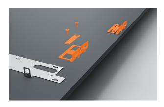
**3.** Align the side brackets to the panel. Secure using the supplied screws. Ensure brackets are fitted tightly and the fasteners are secured straight.
