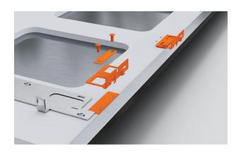
**6.** Align the side brackets to the panel. Secure using the supplied screws. Ensure brackets are fitted tightly and the fasteners are secured straight.
