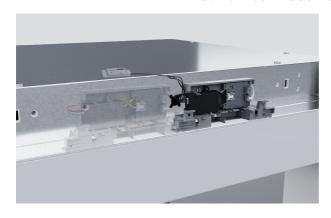
**4.** Move the sensor housing to align the opposite hall sensor clip with the centre of the cabinet
