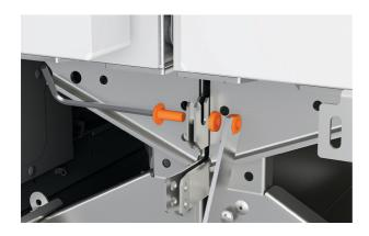
2. Secure the lower brackets together using the supplied M6 screw and Nut. Secure using a 4mm Allen key and 3/8" (10mm) spanner.
