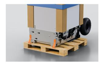
**5.** Removing the remaining brackets.
