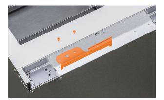
**5.** For the non-hinge side, remove the alcove bracket by unscrewing the M6x16 countersunk screws.
