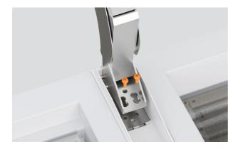
2. Open the centre hinge and reinstall using two M6x16 countersunk screws.
