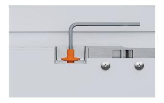
**1.** Ensure top mounting screws have been loosened by 3mm.
