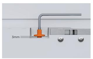
**3.** Loosen the M8 screws by 3mm.
