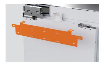
2. Remove the hanging bracket and set aside for later use. Repeat for lower drawer if required.
