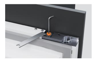
**8.** Tighten the M8 nuts using the supplied spanner and hex key.
