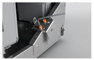
**3.** Re-tighten the cap screws.
