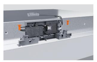
**3.** Remove the two #8x16 screws from the sensor housing.
