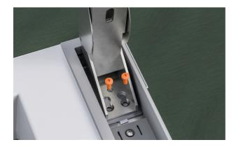
**2.** Unscrew M6x16 countersunk screws to remove upper hinge and set aside.
