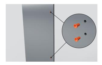
**2.** Remove the four plugs from the door panel.
