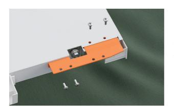
**3.** Install the new upper adapter bracket into the other side of the top of the door with four M5x10 screws.
