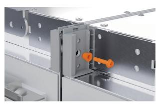
**3.** Clamp the upper brackets together by fitting the first supplied M5 bolt and joiner sleeve. Tighten using a 5/16" (8mm) socket and Phillips screwdriver until the sleeve sits flush.
