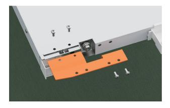
1. Unscrew the four M5x10 screws to remove the upper adapter bracket from the top of the door.
