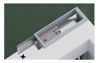
2. Install the new hinge pocket and alcove top bracket on the new hinge side using two M6x16 countersunk screws.
