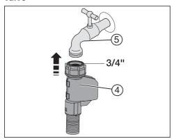
■ Connect the nut ④ to the shut-off valve ⑤.
