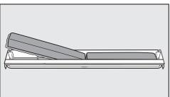
Remove both carbon filters and place the new filters with the surrounding edge pointing downward in the holder.
