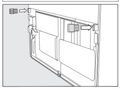
■ Install the wall spacers onto the back of the refrigeration appliance on the bottom left and right.
