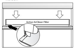
Place the holder in the middle of the protective strip at the back of the adjustable shelf so that it clicks into position. ■ Touch the *OK* sensor control to confirm that the filters have been replaced.
