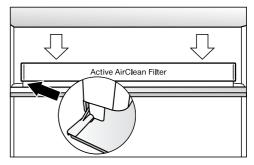
■ Reinstall the holder on the protective strip.
