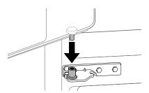
Fit the hinge **1** over the hinge lever latch **2** and slot it into place. Rotate the lever 3 clockwise and fasten the hinge.
