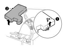
2 Disconnect all wire harnesses **3**. Unscrew the ground wire **4**. Remove the cover.
