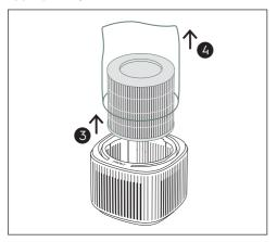
Carefully insert the filter back into the product (either end of the filter works). Make sure that the filter is placed in the center of the cavity.
