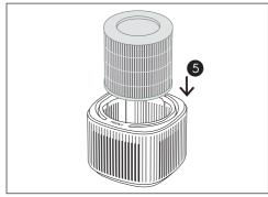
Put back the top part of the main body to close the product till it is securely in place. The mark "FRONT" should be facing the front side of the product.
