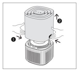
Take out the filter. Carefully remove the plastic bag around the filter and discard appropriately.
