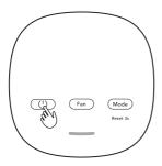
NOTE: When turning ON the air purifier, it will take about 10 seconds for the sensors to calibrate and analyze the air quality. During this time, the air quality indicator will pulsate slowly in white.
