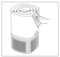
The area around the air inlet on the bottom of the unit may accumulate more dust than some other parts and hence may require more frequent cleaning to ensure optimal performance. The filter is equipped with a mesh filter and should occasionally be wiped off or cleaned with a vacuum cleaner to avoid loss of performance.
