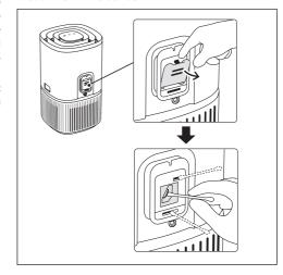
After having cleaned the sensor box, we recommend to vacuum clean the filter at the same time.
