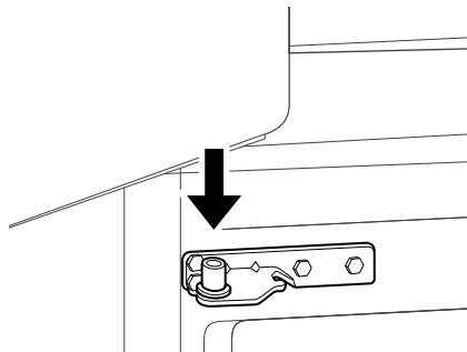
**2** Fit the hinge ① over the hinge lever latch ② and slot it into place. Rotate the lever ③ clockwise and fasten the hinge.
