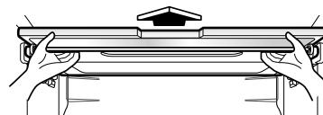
**2** Lift the rear of the shelf slightly and pull it out.
