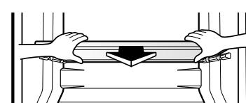
**3** To assemble, slide the shelf into the guides until it stops.
