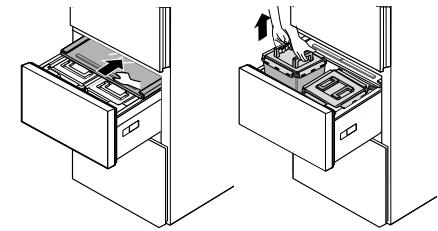
**2** Closing the compartment automatically closes the cover.
