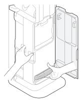
Remove dust from the motor protection filter and exhaust filter once every 3 months and wash it using room temperature water.
